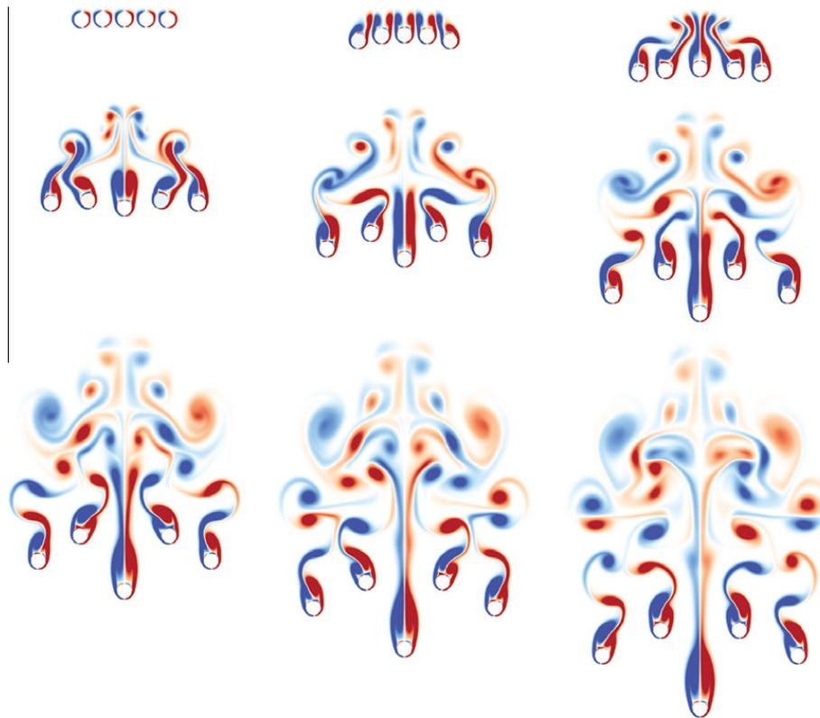
**Fig. 7.** Vorticity plots of five free falling cylinders. From left to right and top-down:  $t = 0.066$  s,  $t = 0.33$  s,  $t = 0.66$  s,  $t = 1.0$  s,  $t = 1.33$  s,  $t = 1.66$  s,  $t = 2.0$  s,  $t = 2.33$  s,  $t = 2.66$  s.
