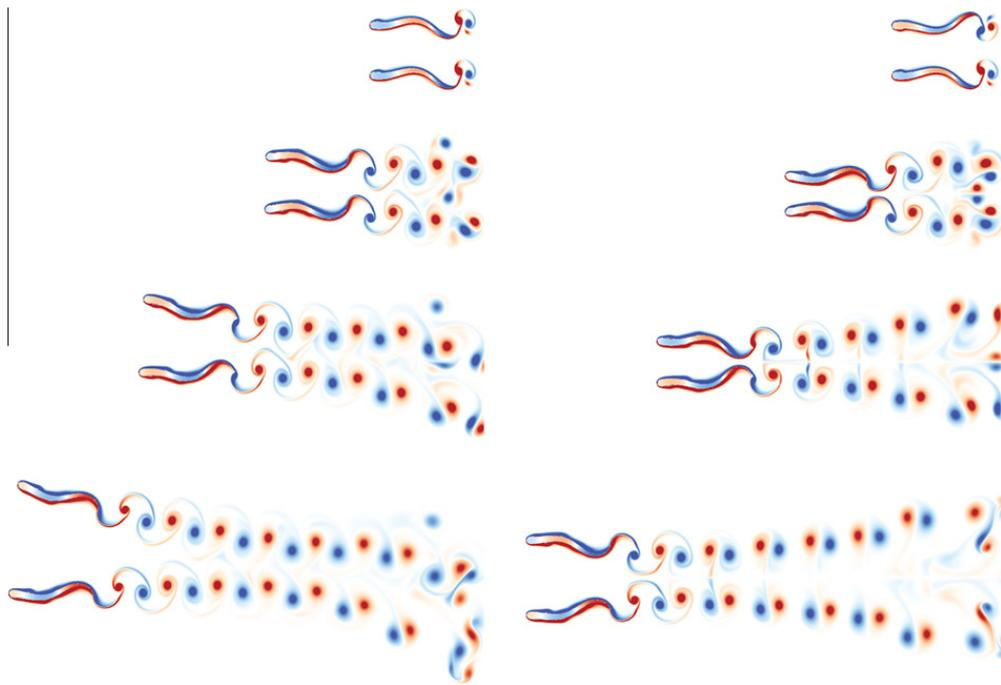
Fig. 18. Tandem fish vorticity plots: (left) phase fish, (right) anti-phase fish. From top to bottom  $t/T = 2.0$ ,  $t/T = 3.5$ ,  $t/T = 6.0$ ,  $t/T = 8.5$ .
