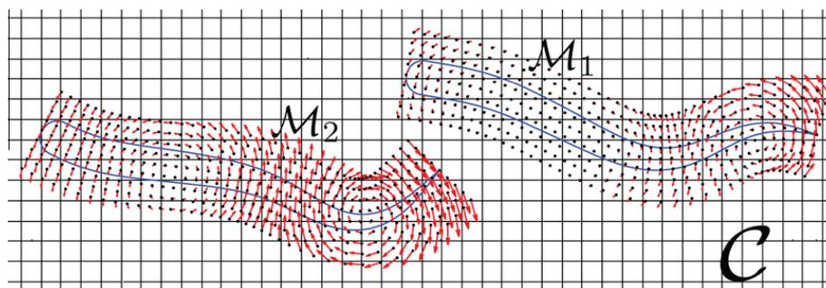
**Fig. 1.** Schematic of the use of the grids. Here two independent shapes are embedded in their corresponding deformable grids  $\mathcal{M}_1$  and  $\mathcal{M}_2$ , that carry the values of deformation velocity  $\dot{\mathbf{r}}_{\mathcal{M}_1}$ ,  $\dot{\mathbf{r}}_{\mathcal{M}_2}$  and characteristic function  $\chi_{\mathcal{M}_1}$ ,  $\chi_{\mathcal{M}_2}$  to be bilinearly interpolated onto the Cartesian computational grid  $\mathcal{C}$ .
