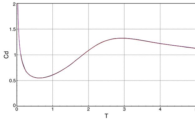
**Fig. 2.** Drag coefficient ( $C_d$ ) at  $Re = 1000$  against the nondimensionalized time  $T$ . The red line is obtained with a resolution of  $2048 \times 2048$ ,  $LCFL = 0.01$ ,  $\lambda = 1e^4$  and  $\epsilon = 2\sqrt{2}h$ . The black and blue lines are, respectively, the reference solutions [47] and [37]. (For interpretation of the references to colour in this figure legend, the reader is referred to the web version of this article.)
