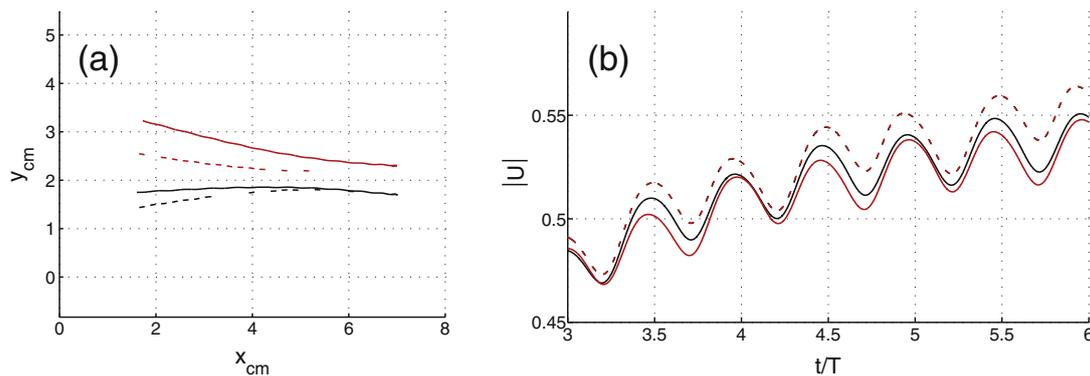
Fig. 19. Tandem fish: (a) trajectories of phase tandem (solid lines) and anti-phase tandem (dashed lines), (b) absolute velocities  $|U|$  of phase tandem (solid lines) and anti-phase tandem (dashed lines). Coordinates and velocities are normalized by  $L$ .
