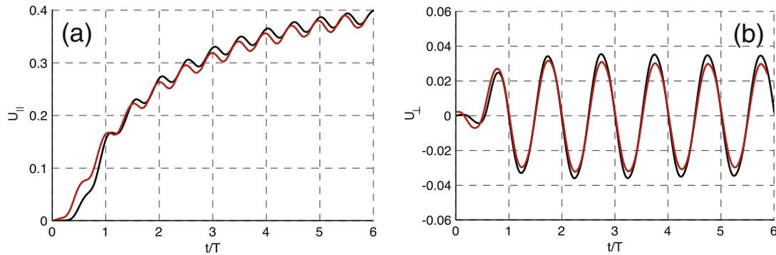
**Fig. 22.** 3D anguilliform swimmer: (a) Forward velocity  $U_{\parallel}$ , (b) Lateral velocity  $U_{\perp}$ . Red lines indicate 3D swimmer simulations with the proposed method. Black lines indicate the reference finite volume solution [22]. (For interpretation of the references to colour in this figure legend, the reader is referred to the web version of this article.)
