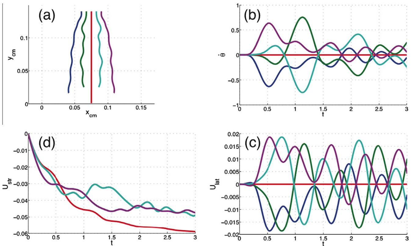
**Fig. 8.** Five free falling cylinders. (a) Trajectories of the centers of mass, units expressed in  $m$ , (b) angular velocities  $\dot{\theta}$ , (c) streamwise velocities, expressed in  $m/s$ , (d) lateral velocities, expressed in  $m/s$ . Time  $t$  is expressed in seconds.
