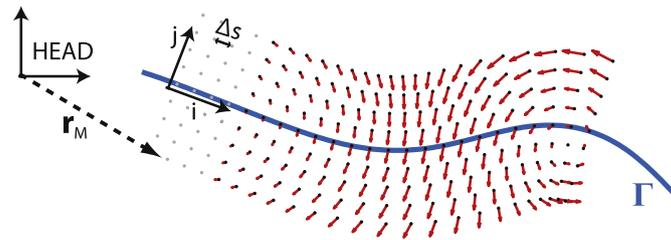
Fig. 25. Deformable mesh and resulting deformation velocity field.
